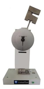
Notched Izod Impact is a single point test that measures a materials resistance to impact from a swinging pendulum. Izod impact is defined as the kinetic energy needed to initiate fracture and continue the fracture until the specimen is broken. Izod specimens are notched to prevent deformation of the specimen upon impact. This test can be used as a quick and easy quality control check to determine if a material meets specific impact properties or to compare materials for general toughness.
