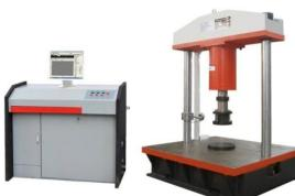
Conform with international standard of *EN 124:1994* Gully Tops and Manhole Tops for Vehicular and Pedestrian Areas-Design Requirements, Type Testing, Marking, Quality Control. GB/T 23858:2009, GB/T GB26537-2011 etc.,
